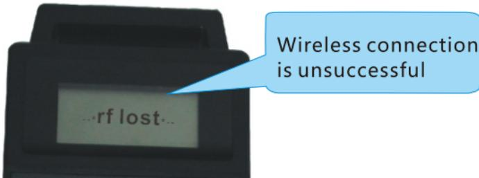
When the wireless USB receiver is connected MPG and unsuccessful (eg USB receiver does not plug in the computer), the wireless MPG's LCD will appear as follows:
