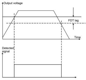
Figure 5 - 09 FDT level diagram
