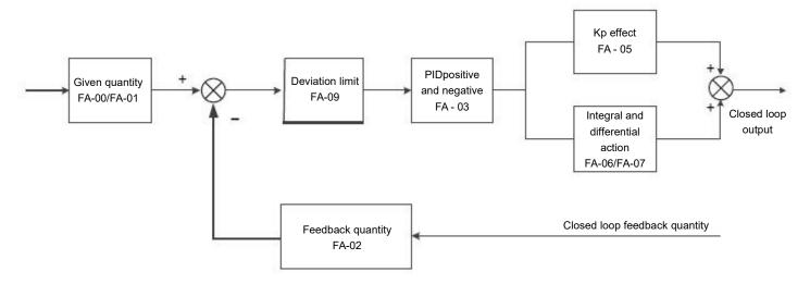
Figure 5 - 27 process PID principle block diagram
