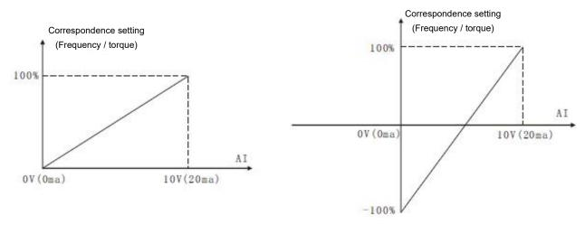
Figure 5 - 16 simulates the correspondence between a given value and a set value
