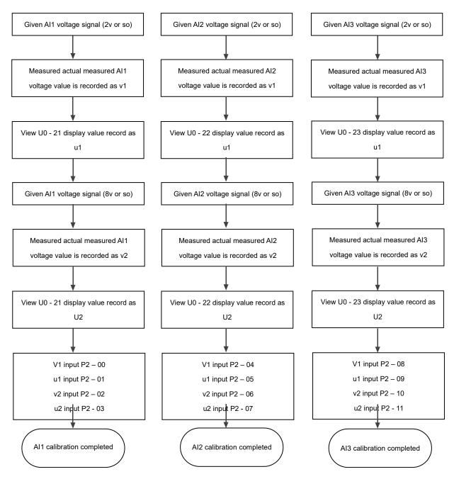
Figure 5 - 34 Al calibration method diagram
