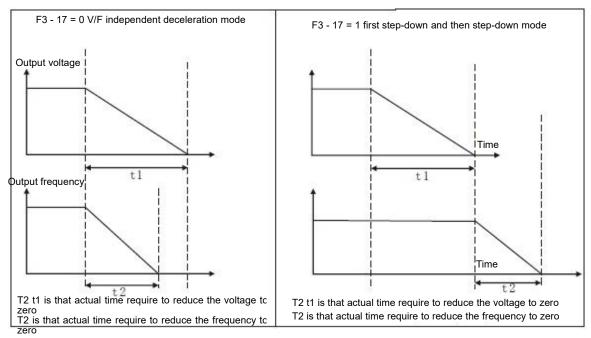
Figure 5 - 07 V/F separation shutdown process diagram
