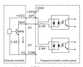
Leakage (NPN) connection mode
