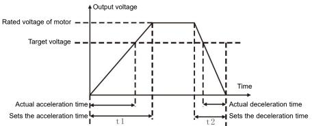
Figure 5 - 06 V/F separation diagram
