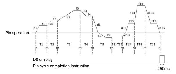
Figure 5 - 31 simple PLC operation diagram
