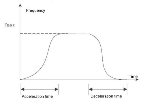
Figure 5 - 21 S curve acceleration and deceleration
