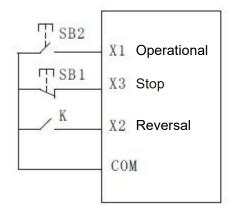
Figure 5 - 15 three-wire control modes 2
