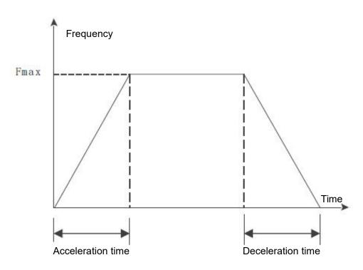
Figure 5 - 20 linear acceleration and deceleration
