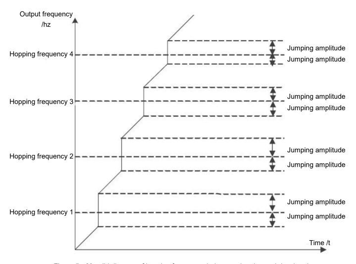
Figure 5 - 23 valid diagram of jumping frequency during acceleration and deceleration
