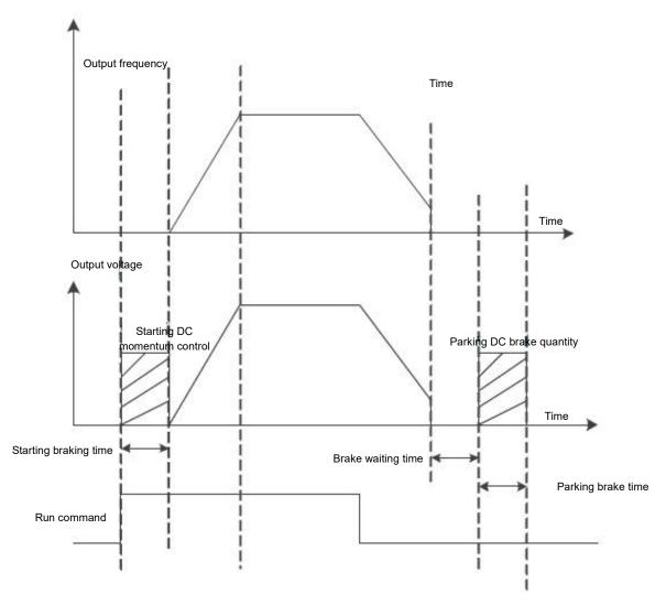
Figure 5 - 19 schematic diagram of DC braking
