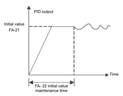
Figure 5 - 30 functional diagram of PID initial value
