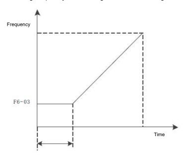
Figure 5 - 18 startup frequency and startup time
