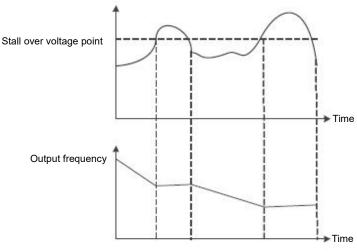
Figure 5 - 26 over voltage stall function
