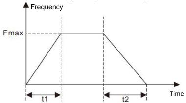
Figure 5 - 1 schematic diagram of acceleration and deceleration time
