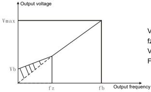
Vb: manual torque lifting diagram (lifting amount is shaded part)
