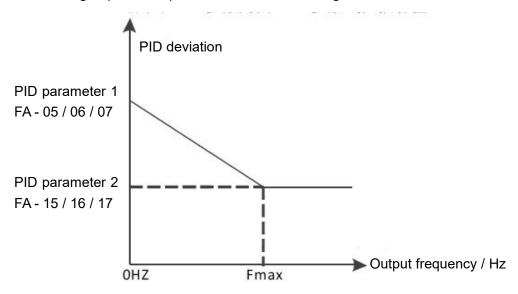
Figure 5 - 29 schematic diagram of PID switching according to operating frequency
