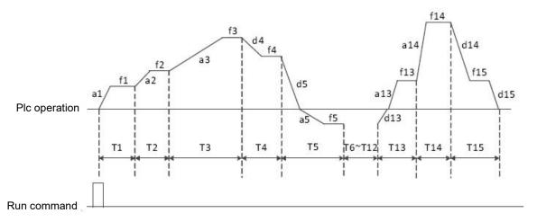
Figure 5 - 32 shutdown modes after single cycle
