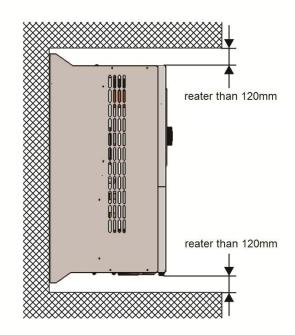
Monomer installation: the size of A is larger than 150 mm, because the upper and lower directions are air ducts, the space distance should be increased.
