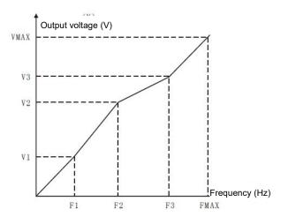
Figure 5 - 05 multi-point V/F curve setting diagram
