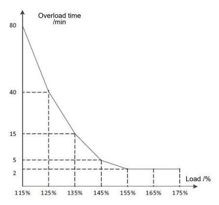
Figure 5 - 25 overload current vs. overload time curve
