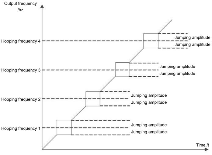
Figure 5 - 22 Hopping frequency diagram
